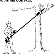
Keep a good, firm grip on the pruner with both hands when the engine is running and don't let go. A firm grip will help you reduce kickback and maintain control. Keep the fingers of your left hand encircling and your left thumb under the assist handle. Keep your right hand completely around the
